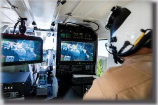
From startup, taxi, and operations over the target area, the VCTS replicates the look and feel of todays Airborne Law Enforcement aerial support platforms. With outside views in spectacular 4K resolution and wrap-around visibility up to 240° using 3-channel COTS projection system that delivers a truly immersive experience.
